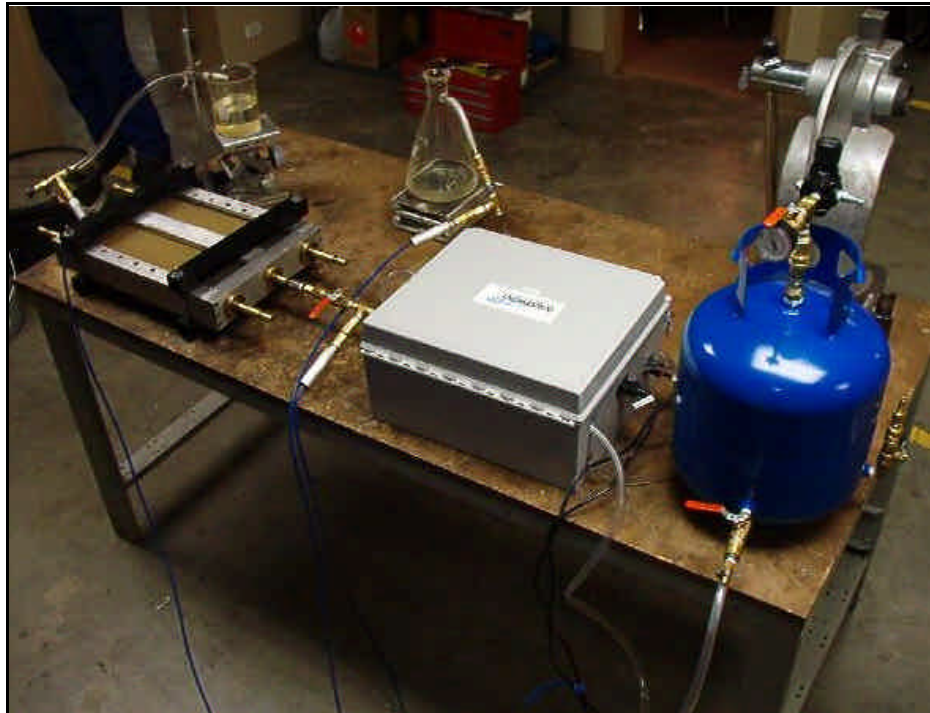
Figure 7: The pulser here consists of a tank containing fluid at a fixed pressure. A solenoid is opened causing the pressurized fluid to enter the cell over a 10^{\text{th}} of a second. That solenoid is then closed and another solenoid is opened allowing the pressure to go back to ambient conditions over a period of a second.
