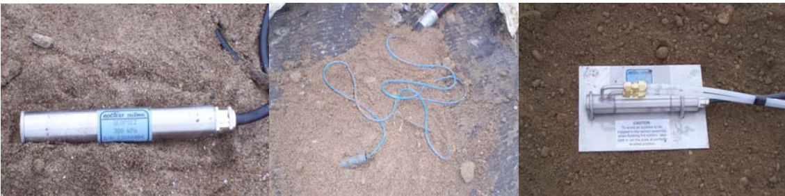
Figure 5. Sensors to measure leachate level, temperature and settlement
