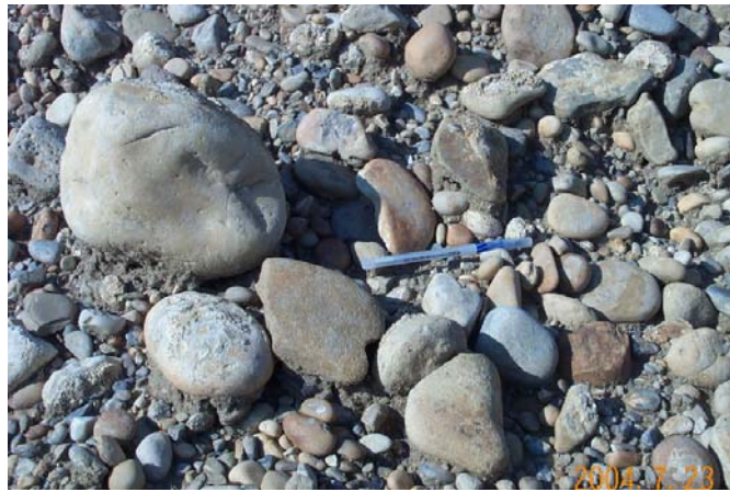
Figure 4: In-Situ Soil at 11-17 (Note the Size of the Pen and Coarse Material)
